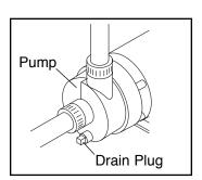
until all the water has drained from the pump. Replace the drain plug.
